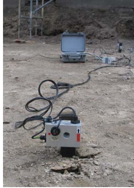
Figure 3.5 Photo of triaxial geophone (foreground) and the recording device (background) from the Karlstad theatre field test.
